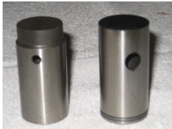
1951-54 V-8 lifters. To the left is for cast Iron cams, the one to the right for forged steel cams
