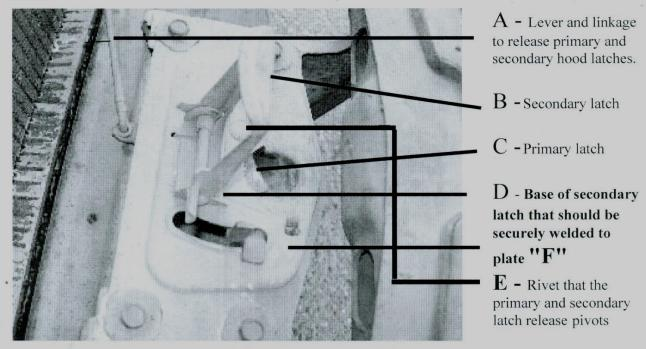
A bolt may be used to secure the base of the secondary latch to plate F. If this is to be attempted, one must make sure that it will not restrict the movement of the latch release mechanism as it pivots from rivet marked "E." To ensure that the nut does not come loose, use either LocTite or self locking nut. Suggested bolt size to be 5/16". Locate it so that it does not restrict movement of the latch operation.
