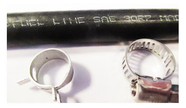
The picture shows hose/fuel line with SAE 30R7, rated for cars with carburetors. Also, pictures are hose clamps. My preference would be the screw clamp on the right. There are different hose clamps for fuel systems that exceed 50 psi.
