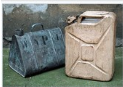
German containers for 20 litres of fuel. left: former container, right: Wehrmacht-Einheitskanister of 1941, manufacturer: Nirona
