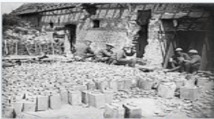
British pressed steel, 2-imperial-gallon (9 l) petrol cans: Strong, but heavy and expensive
